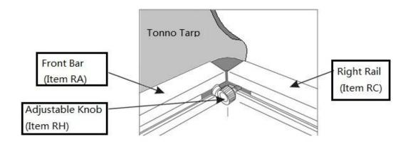
5. Attach front bar & cover assembly by inserting corners (Step4), Align frame from front to rear and side to side.
