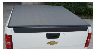
10. To open the cover, open the truck bed tailgate, pull the handle in the middle of the cover Rear Bar, unlock the bar, roll up the whole cover to the front of truck bed, then use the buckles to secure the rolled tarp.
